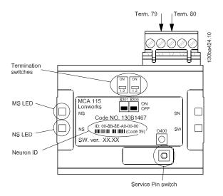
The LonWorks option is equipped with two termination switches, S300 and S301, enabling double termination when using bus topology.
