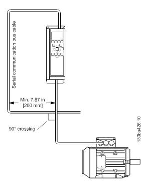
It is highly recommended to use suitably shielded cable for any LonWorks installation!
