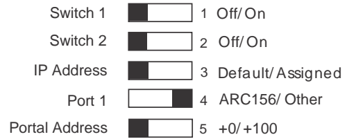
Figure 15. BACnet Portal DIP Switches
