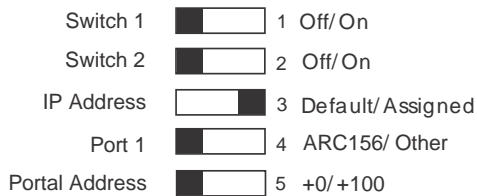
Figure 7. BACnet Portal DIP Switches
